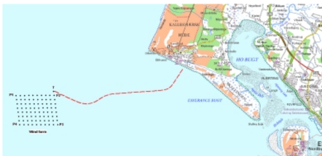
Figure 2.1 Location of offshore wind farm and cable to shore. The substation is located at the T.
